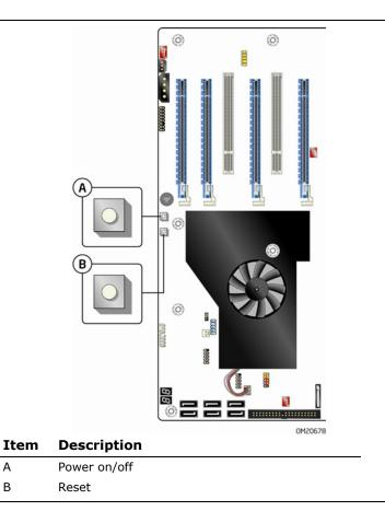
Figure 8. Location of the Onboard Power Button
